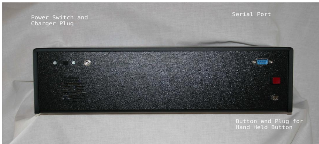
KitST Rear showing switches and connectors.
